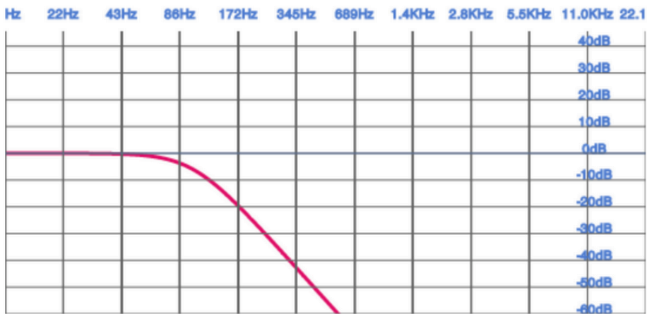
Figure 6-1. Frequency response graph for a low-pass filter
